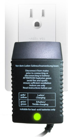
Green indicates charging complete
