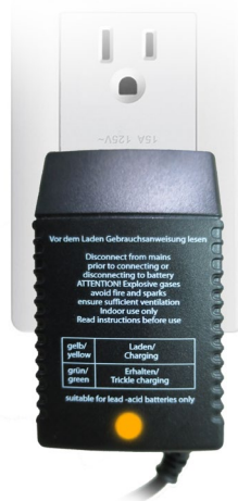
Yellow indicates charging
