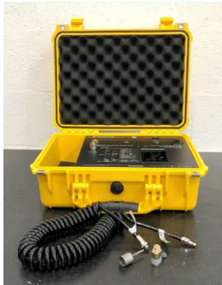
Use the Ayrton IP TEST KIT to control the IP rating of the fixture.
